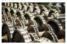
**BONASTAR®** is a family of enhanced wheel steel grades for all types of passenger, locomotive and freight wheelsets. In comparison with wheels made of common grades, **BONASTAR®** ensures significantly greater life in mileage.
